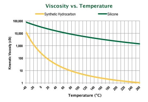
A Note on Viscosity Index (VI) The viscosity of an oil gets thicker at low temperatures and thinner at higher temperatures. Viscosity Index indicates how much viscosity changes from -40°C to 100°C. High VI indicates small viscosity change, as in the silicone plot above. Low VI indicates large viscosity change with temperature. High VI ensures more consistent part performance over wide temperature ranges.
