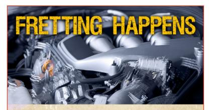
Fretting wear is also known as vibrational wear. Because virtually all machines vibrate, fretting is likely to occur:
